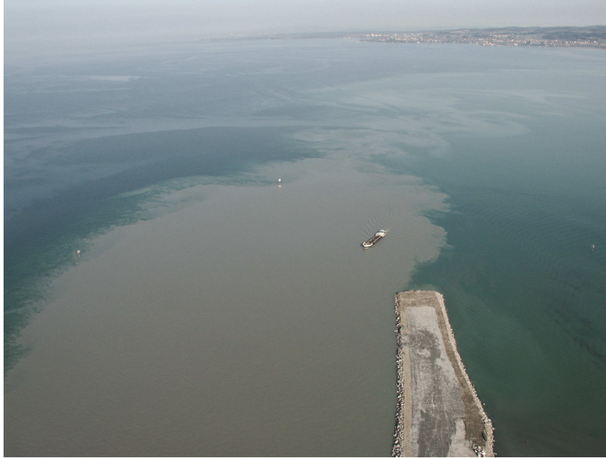
Figure 2: Close-up to the mouth of the river Rhine (Alpen-Rhein) at Fussach, near Bregenz, showing the right river dam and the suspended sediments (wash-load) with the strong spatial variation of its concentration. Copyright: ‘Tino Dietsche - airpics4you.ch ’
