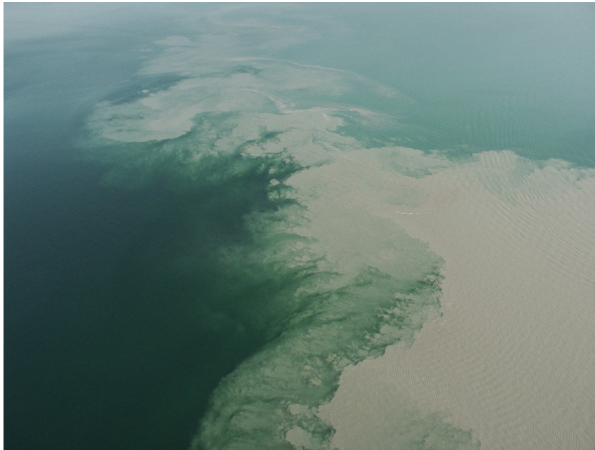
Figure 13: Sediment laden water in the forefront of the estuary mouth of the river Rhine (Alpen-Rhein) at Fussach near Bregenz, Austria. The picture demonstrates that up-welling and down-welling processes must be active, indicating that the Shallow Water Approximation in computational software should not be applied. A full non-hydrostatic three dimensional model is required. Copyright: ‘Tino Dietsche - airpics4you.ch ’
