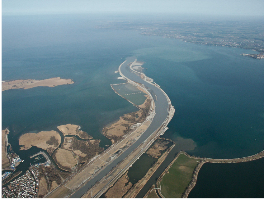
Figure 1: Channelized entrance of the river Rhine (Alpen-Rhein) into Lake Constance at Fussach, near Bregenz, showing alternating sandbanks within the artificial channel and a large patch of suspended sediments in front of the river mouth. The island on the right frame is Lindau. Copyright: ‘Tino Dietsche - airpics4you.ch ’
